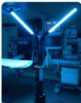
UV Disinfection System
