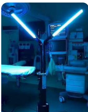
UV Disinfection System
